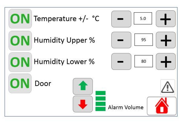
The Alarm Set Screen can be used to configure the setpoints for various process alarms in the incubator, including temperature, humidity, and door state.
