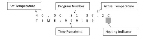
F. When the unit is in full heat mode, a white square on the far right of the lower display line will illuminate. When the heater is maintaining temperature, the white square will flash. When the heater is off, the white square is no longer illuminated.
