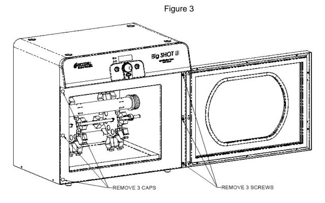
8.1 The door on the hybridization oven is reversible for visibility. To change the doors position simply remove the 3 screws & 3 caps as show in figure 3. Using the same screws reposition the door to the side desired, be sure that all screws are secured properly. Place the caps in the unused holes that the hinge previously was mounted to.
